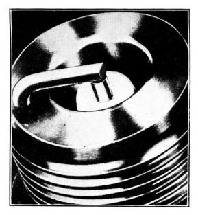
Shows a clean and efficient sparking plug.
