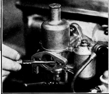
The correct way to adjust the carburetter is to set it correctly at its idling speed. The carburetter is then set throughout its range. This adjustment is made by means of the jet and the jet adjusting nut; in other words, the position of the jet is altered relative to the needle.
