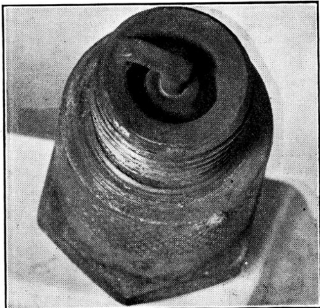
Above is shown a plug which has become fouled by a dry, fluffy black deposit and indicates faulty carburation or a defect in the ignition system.
