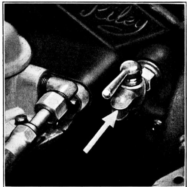
Right.—The location of the cylinder block drain tap just forward of the fuel pump.
