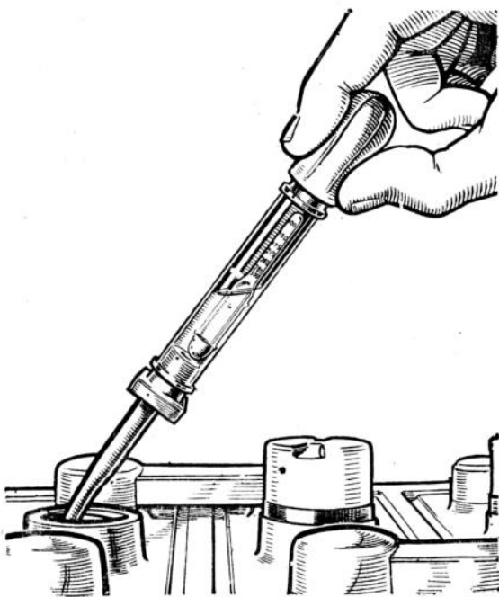
Above.—Top-up the battery with distilled water.
