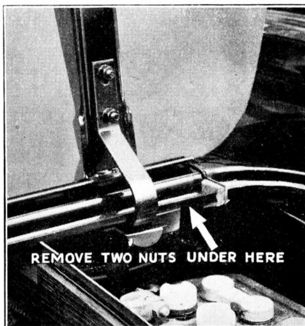
Above.—At the rear end of, and underneath, the centre panel are two nuts which must be removed prior to detaching the complete bonnet.
