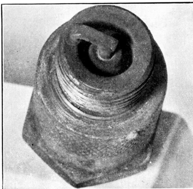
Above is shown a plug which has become fouled by a dry, fluffy black deposit and indicates faulty carburation or a defect in the ignition system.
