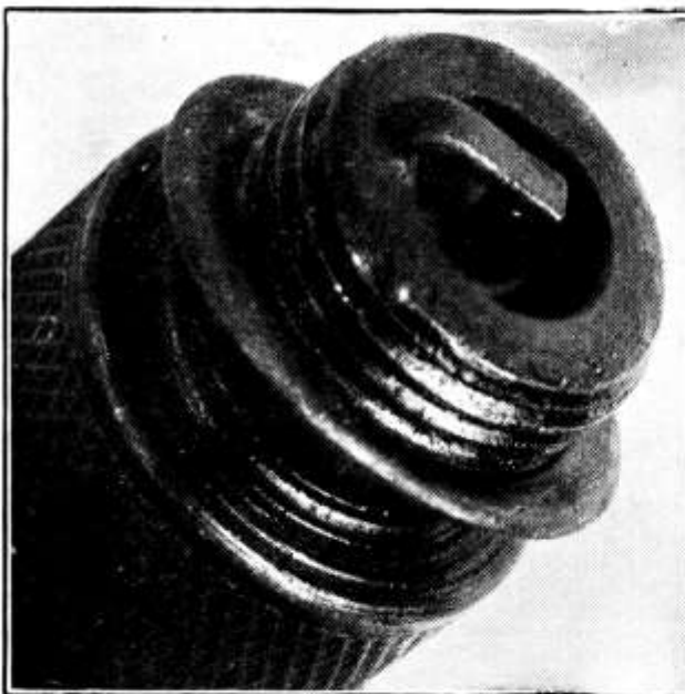
This plug shows signs of oil-fouling, indicated by a wet, shiny black deposit on the insulator. This type of fouling may be caused by worn pistons, cylinders or gummed-up piston rings.
