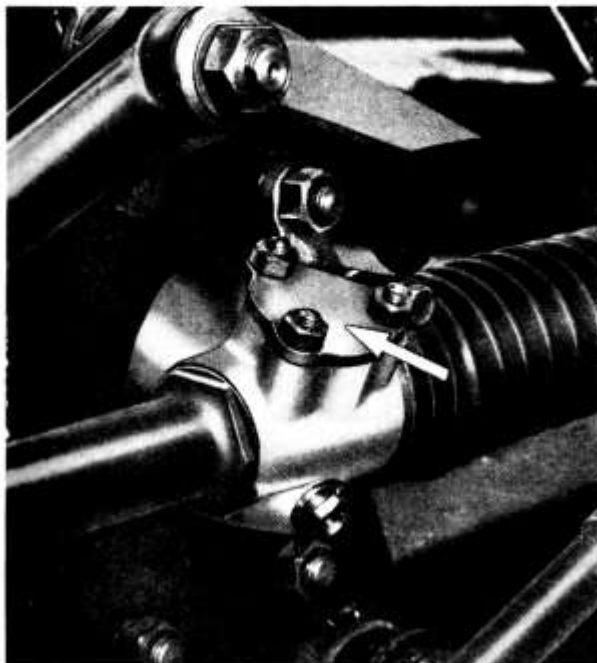
Left.—The arrow indicates the plunger housing, which must be removed prior to greasing the steering gear.
