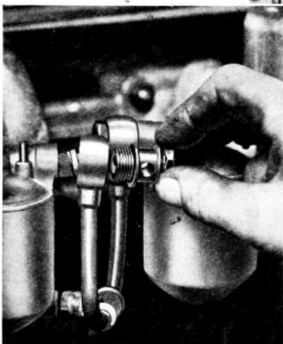
Left.—Shows one of the carburetter filter assemblies. Note the correct positioning of the filter and spring with the open end of the filter outwards. The banjo bolt has had the washers reassembled in their correct relative positions, i.e. one either side of the union. Make sure the washers are perfectly clean when reassembling.
