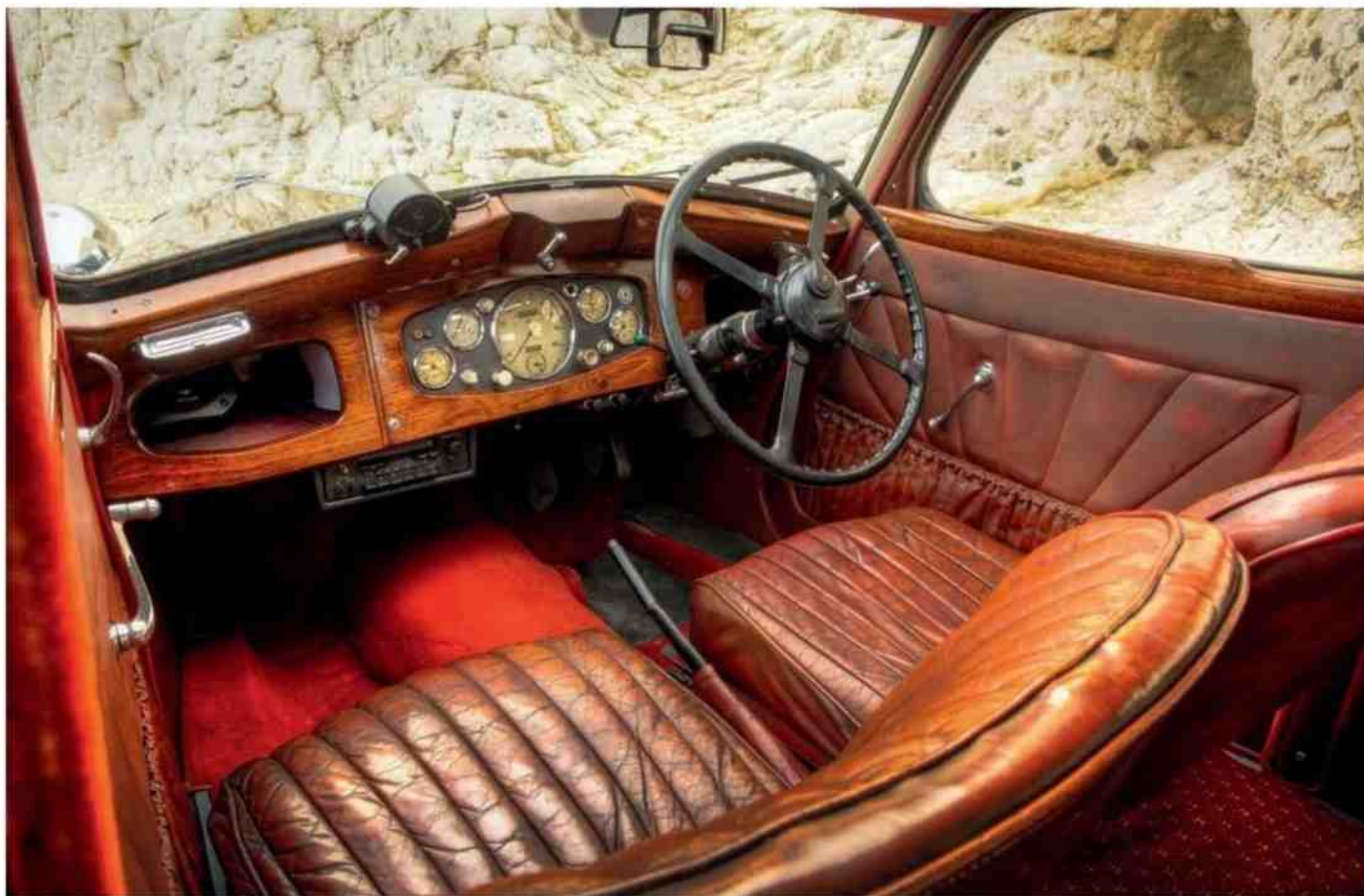
Clockwise, from above: cossetting interior – seats would originally have had pneumatic cushions; simple detailing; Riley was in the midst of one of its most prolific periods when it launched the 12/4; deceptively small boot is accessed via a split lid
