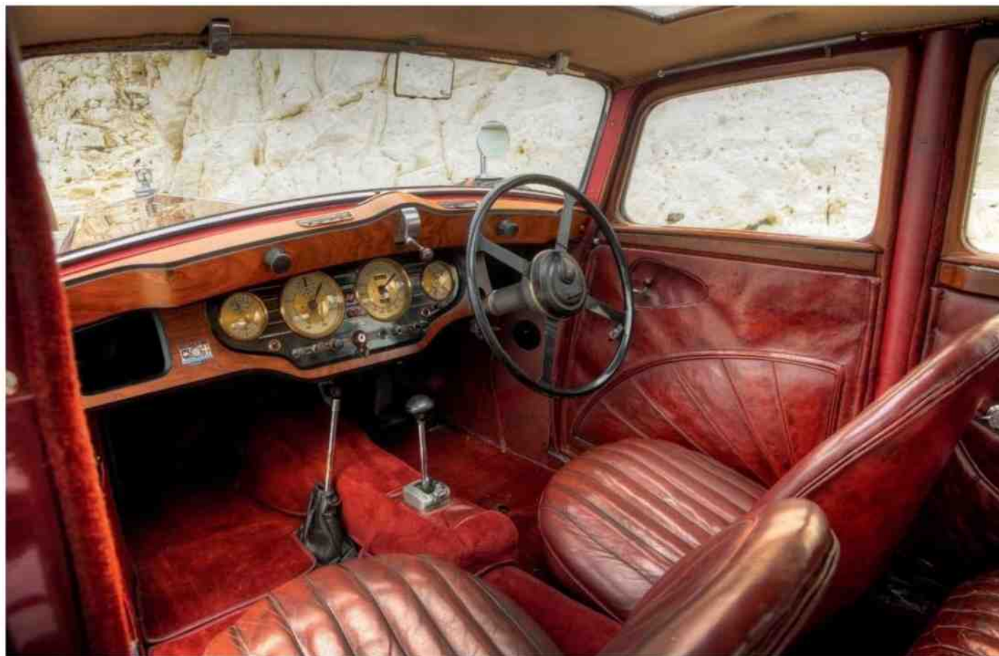
Clockwise, from above: gorgeous interior boasts a well-organised dashboard – this pre-production model features a fly-off handbrake; neat MG motif on doorhandles; radiator-mounted temperature gauge is a later addition; substantial rear end
